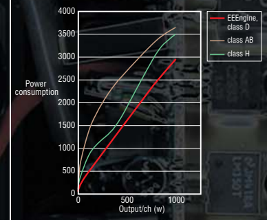
Figure 3: Efficiency comparison data (power consumption vs. output)
