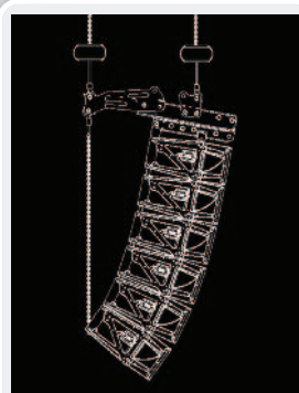
Array angles realised after lifting
