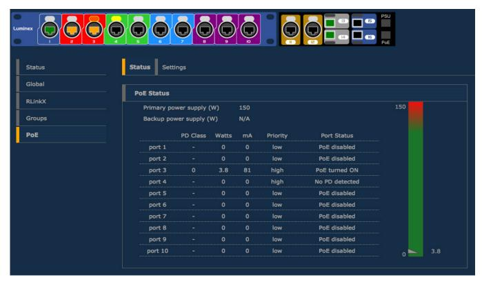
As the V2 firmware now unleashes the optional PoE output power to 150W, the power level bar has been increased up to 150W.
