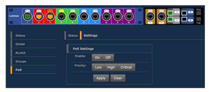
The reset button label has been replaced by a "Clear" label. This button still clears up the ports selection
