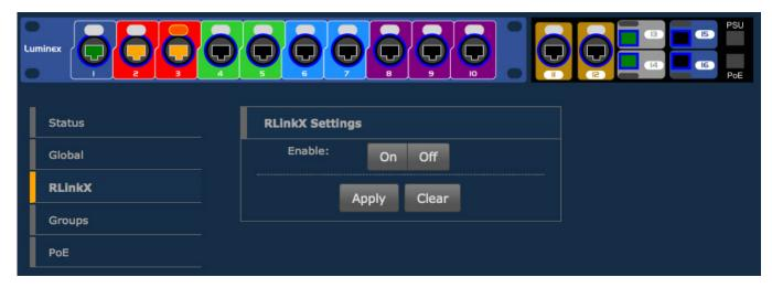
The reset button label has been replaced by a "Clear" label. This button still clears up the ports selection
