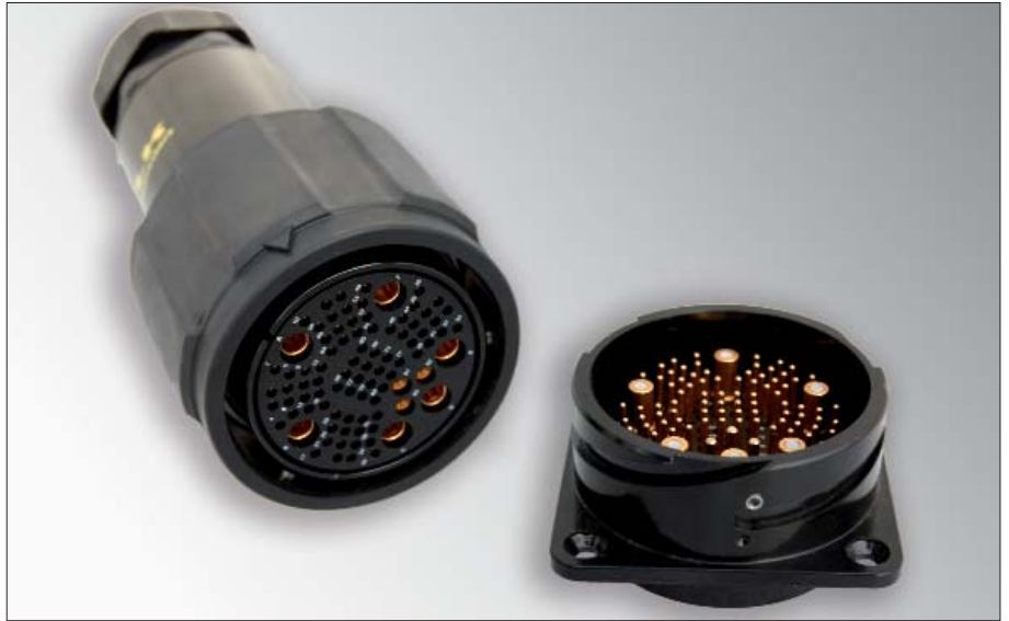
LKA 40/89: 80 pins size 18 for signal transmission, 6 coaxial pins, 3 pins size 12 for power. To obtain improved performance they may be used with many eurocable hybrid cables.
