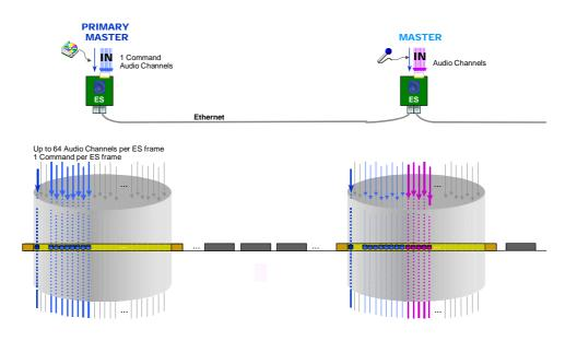
**Notes:** A Master device is always located downstream of a Primary Master device.
