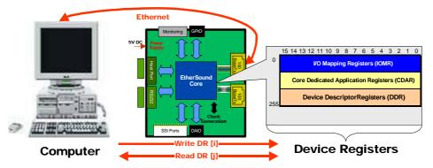
• By software, using the Host Port from an external µController or a DSP. This solution allows reading and writing in any local Device Register. Furthermore, the Host port of the Primary master allows to access any register of any device.
